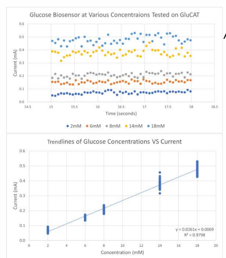
Chronoamperometry Tests: 5 glucose solutions: 2, 6, 8, 14, 18 mM
