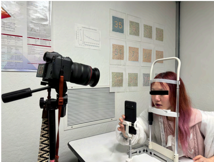
Figure 6. Equipment setup for collecting human lips dataset
