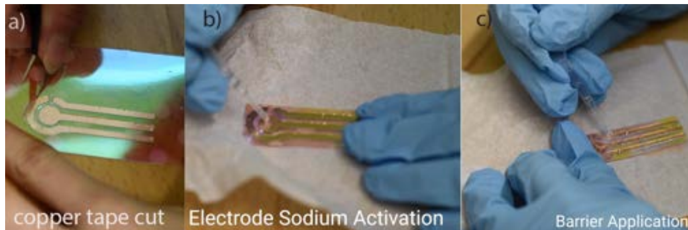
Figure 2: Electrochemical biosensor fabrication process: a) Copper tape cut by the vinyl cutter. b) Sodium activation solution is applied. c) Barrier solution is applied.
