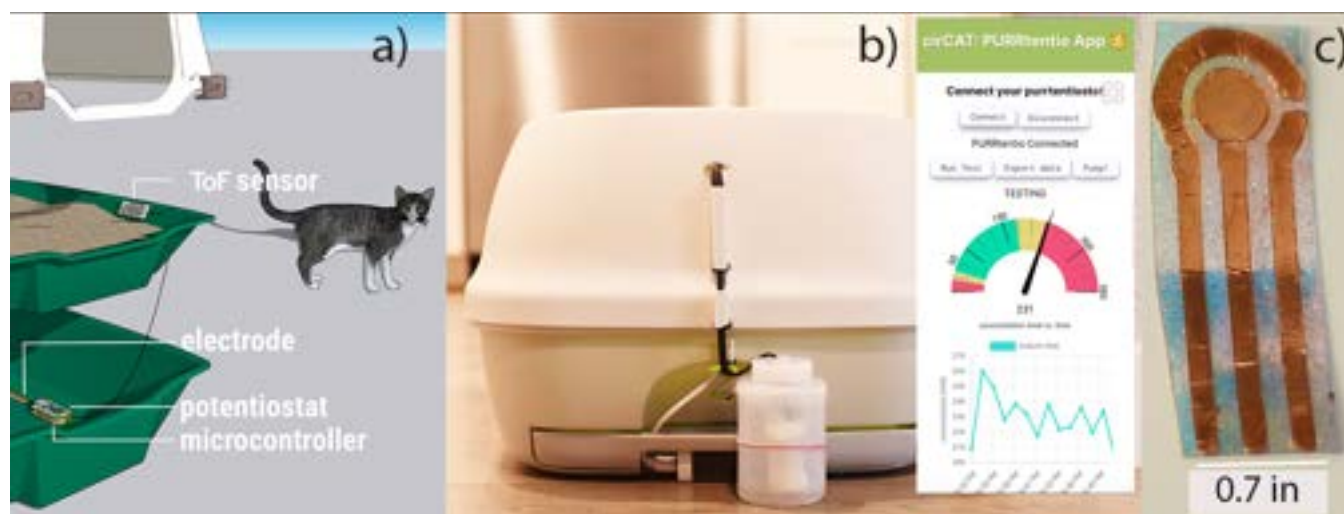
Figure 1: PURRtention a) System components. b) Litter Box System and mobile application readouts. c) DIY electrochemical biosensor
