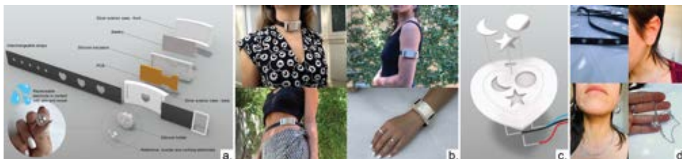
Figure 1: BioSparks: a. System components, b. Modularity, c. Interchangeable electrode, and d. Repurposing
