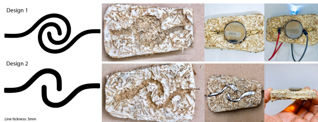
Figure 3: Design 1: Coin battery embedded in mycelium. Design 2: Gallium used on a myco-composite circuit.
