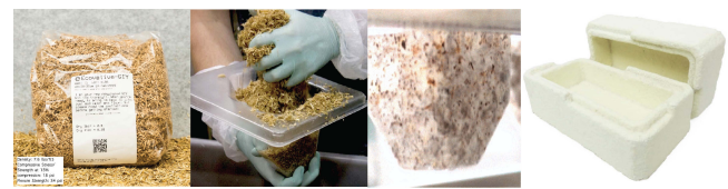
Figure 2: GIY bag and growing mycelium process. Photo: CC0 Ecovative Design.
