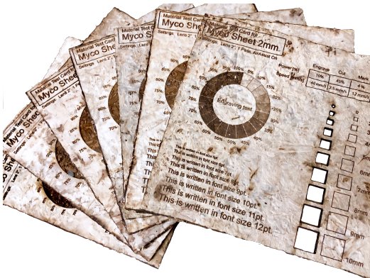
Figure 4. Mycoboard test cards laser cut in different thicknesses.
